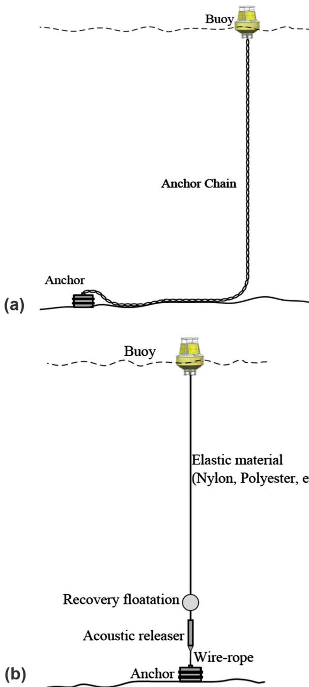
**Fig. 1** (a) Catenary mooring, and (b) Semi-taut mooring [2]
