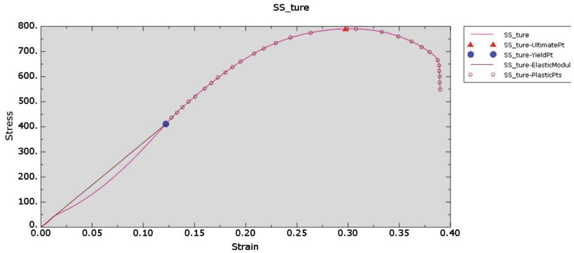
Fig. 9 Tensile properties of R3 steel generated from ABAQUS
