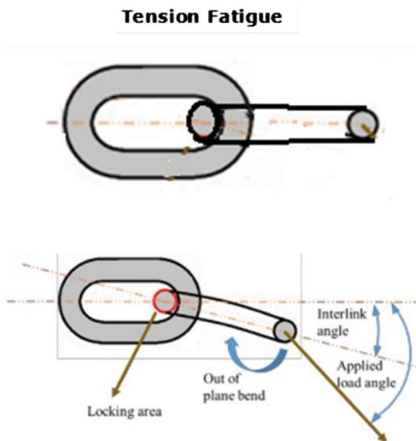
**Fig. 3** Tension fatigue vs Out of Plane Bending (OPB) mechanism [10]
