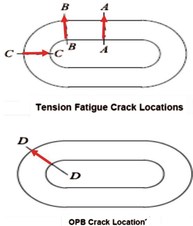
**Fig. 2** Crack locations for Tension vs OPB Loading [10]
